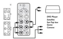
Connect to AV 1,AV 2: Composite (1)+(2), (1)+(4) Connect to AV 1:S-Video (3)+(2) Select source AV 1 or AV 2
